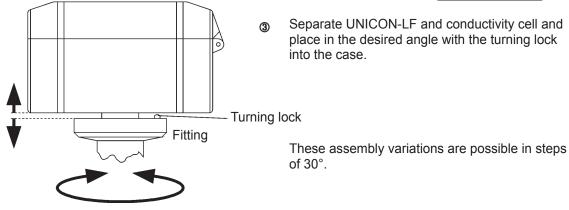
Tighten the Lock nut and Armature of the UNICON-LF.
