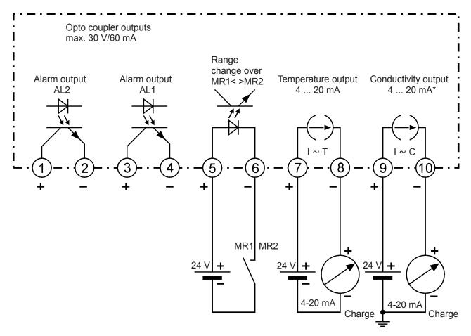
\*For supplying the converter use terminals (9) and (10) as shown. If the converter is used for monitoring only, terminals (9) and (10) must be connected direct to supply voltage.
