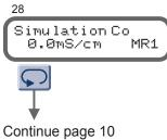
Simulation of the conductivity (manual operation) The converter works as simulator. The output current changes in range 4 ... 20 mA in accordance with the conductivity value set. Setting possible in the preselected measuring range with buttons 🔺 and 🔽.
