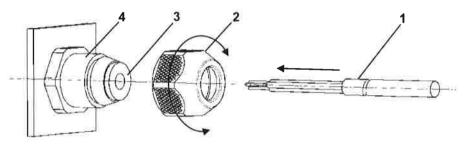
Figure 10: PG / cable screw fitting connection
