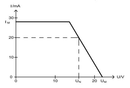
Fig. 5: Transmitter feed, characteristic curve
