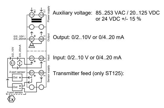
Fig. 3: Connection diagram
