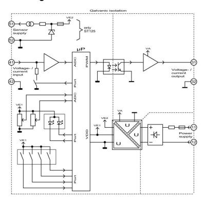
Fig. 1: Block circuit diagram
