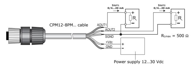
Fig. 3.4: current analog outputs connection
