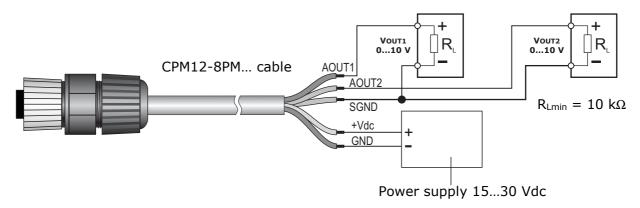
Fig. 3.5: voltage analog outputs connection
