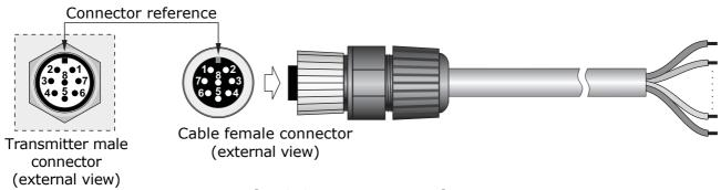
Fig. 3.2: connectors pinout
