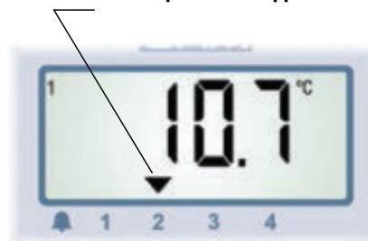
Alarm 2: temperature > upper threshold
