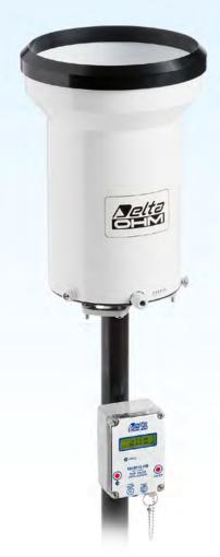
The HD2013 is a reliable and sturdy tipping bucket rain gauge, built entirely from corrosion resistant materials in order to guarantee its durability. So as to ensure accurate measurement even with low temperature climatic conditions or during and after precipitations of snow, a version with heating which is automatically activated around +4 °C has been developed so that snow deposits and ice formations are prevented.
