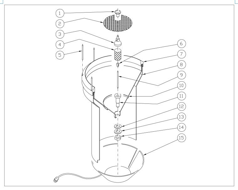
Fig. 13 – Exploded view of the upper part (version with heating)
