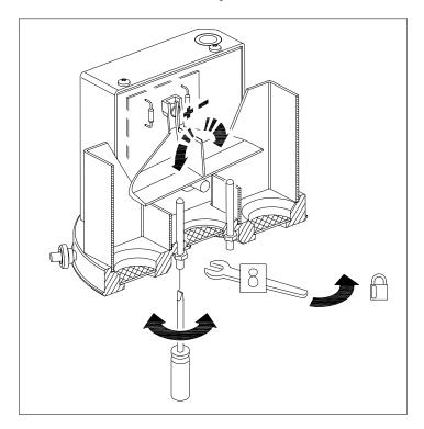
Fig. 7 – Adjustment of the tipping bucket
