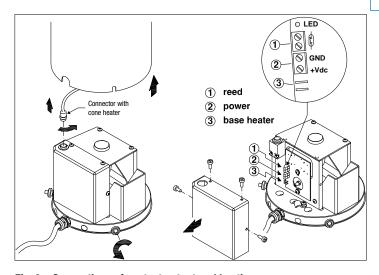
Fig. 2 – Connections of contact output and heating
