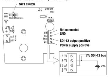
Fig. 4 - Connections of SDI-12 digital output
