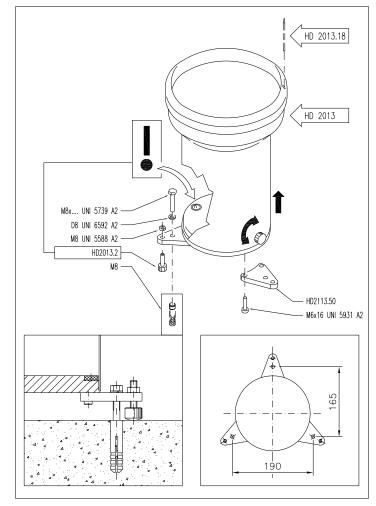
Fig. 10 - Ground installation
