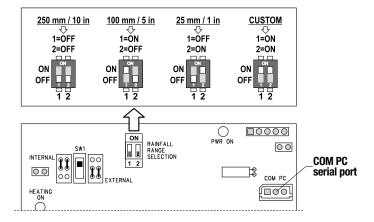
Fig. 5 - Dip switches
