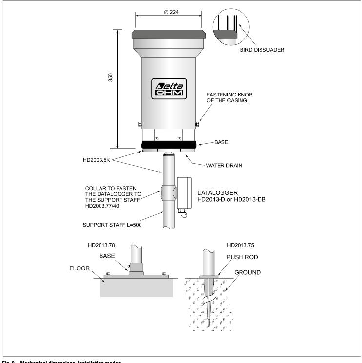
Fig. 8 – Mechanical dimensions, installation modes
