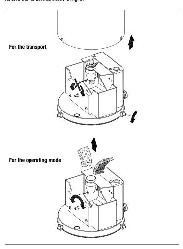
Fig. 6 - Locking and unlocking the tipping bucket
