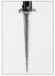
$\label{thm:condition} \mbox{Tip for ground for rain gauge raised from ground}$
