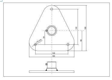
Fig. 9 – Base for ground fastening (HD2013.78)
