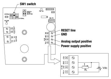
Fig. 3 - Connections of analog output
