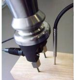
Reciprocating piston electrode GHE91 with temperature-probe GTF38
