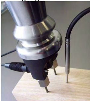
Reciprocating piston electrode GHE91 with temperature-probe GTF38
