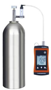
1. If you would like to perform a calibration with test gas, connect the extraction device to the product first.
