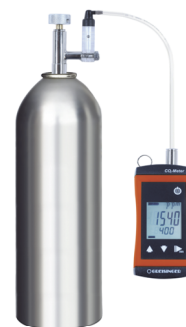
Check with test gas
