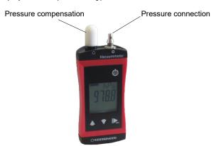
The G1111-xx-VAC has a pressure connection and a pressure compensation. This means that no dangerous internal pressure can build up during evacuation and on the other hand no particles can enter the inside of the device when the vacuum is released, as the pressure compensation element acts as an extremely fine pore filter.
